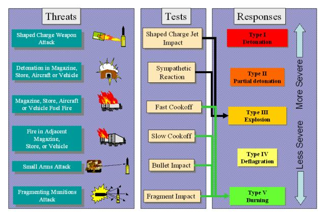
Figure 10 – Tests and reaction Levels [10]
