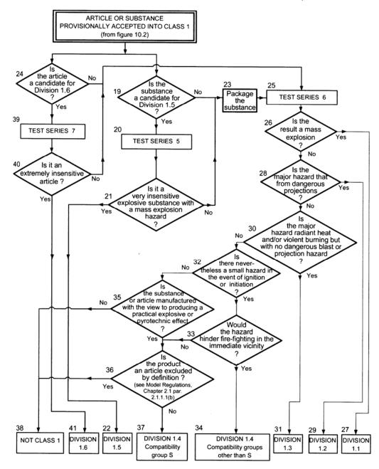
Figure 2 - Class 1 Division Assignment Schematic (Figure 10.3) from UN ST/SG/AC.10/1/Rev.14
